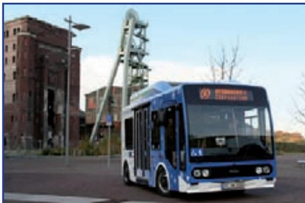
The region of the Emscher-Lippe rivers is home to two vehicle outfitters and the supplier of hydrogen for the project. In Gladbeck, Italian electric buses are equipped with an advanced fuel-cell powered drive by Hydrogenics Ltd.
